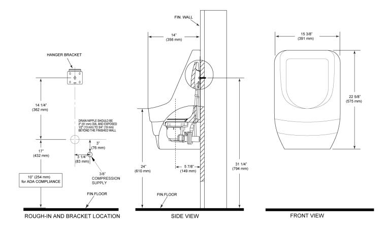
NOTE: ADA urinal rim height requirements allow all heights 17" and below. Strongly recommend roughing in the drain to achieve a 16½" rim height or less to ensure compliance.
