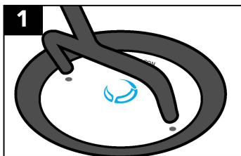
1 Insert key into cartridge.
