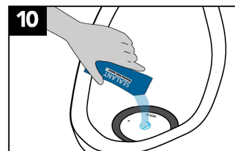
10 Add blue sealant (allow time to drain into cartridge).
